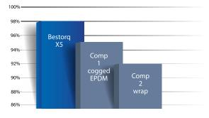
Savings calculation below uses a 20HP, 3-phase, electric motor, and the national average rate of \$0.121/kw-hr, 5.75" driver diameter, and 4 BX or B belts at \$48/set.  $8760 \text{ hr} \times 15 \text{kw/hr} \times \$0.121 \text{ /kw-hr} = \$16,000 \text{/yr}$
