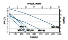
WGFP-33 (2500 GPH @ 5') WGFP-50 (4280 GPH @ 5') WGFP-75 (4890 GPH @ 5') WGFP-100 (6400 GPH @ 5') WGFP-150 (9750 GPH @ 5')
